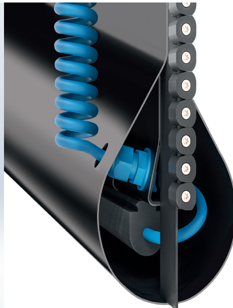
Bottom edge detection via intrinsic safety barrier
