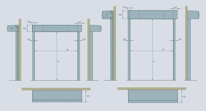
All indicated dimensions are net: the space necessary for mounting and maintenance has to be provided.
